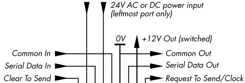
*Wiring of one SMARTPAX port. Power can be supplied to SMARTPAX through the leftmost of the four ports (front view). Most devices are not capable of supplying power to the SMARTPAX, however. Thus, in most cases, a separate power supply is required.*
