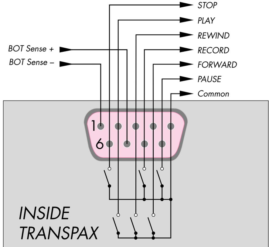
Wiring diagram for the
