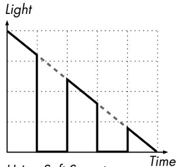
*Using Soft Snap to create a flash-fade.*
