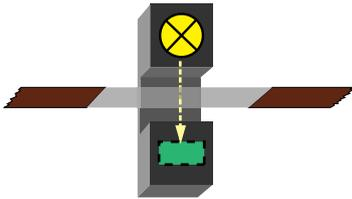
*A transmissive beginning-of-tape sensor.*
