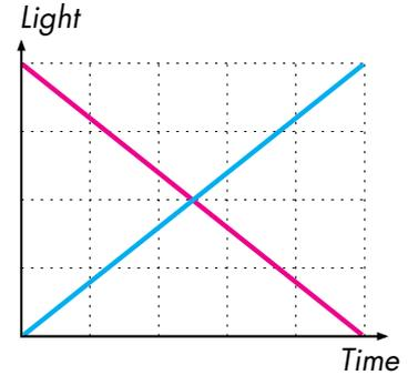
*Linear fading using a Set/Fade cue.*
