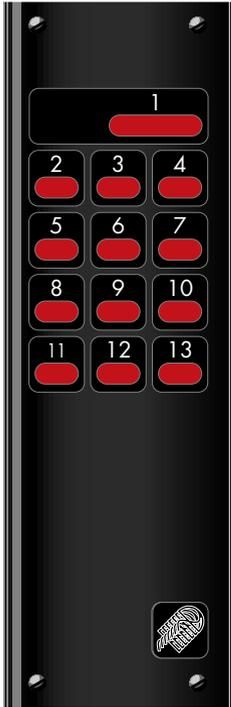
*Numbering of AIRLINK buttons when connected through a SMARTPAX port.*
